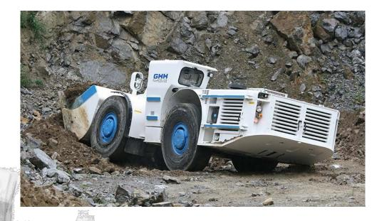
fully hydrostatic version hydraulic motors "in line"
