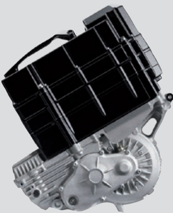
Fully integrated PMS Motor of KTM E-Enduro Freeride-E
